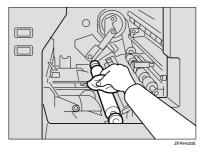
4 With a clean cloth, remove any ink that has accumulated on the trailing edge of the drum unit.
